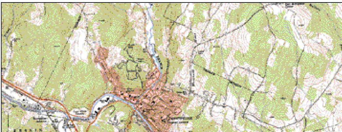
A digital raster graphic image depicting a portion of the Montpelier, Vermont, 1:24,000-scale quadrangle.
