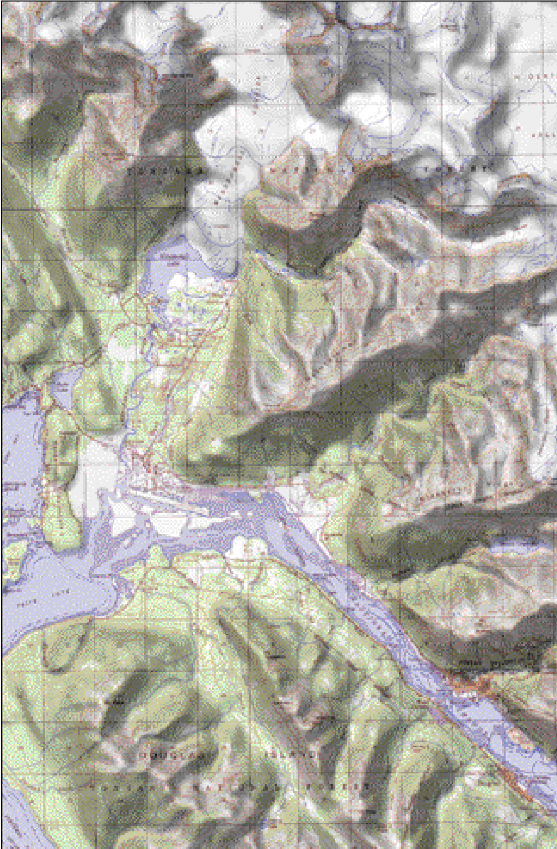
Example of a shaded-relief digital raster graphic showing a part of the Juneau, Alaska, 1:63,360-scale DRG combined with digital elevation model data. This image is intended
