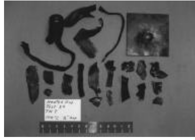
HGT-39. TNT, 0.5-inch gap, 100°C.
