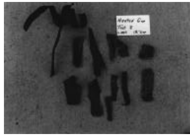
HGT-8. TNT, 1.5-inch gap, 100°C.
