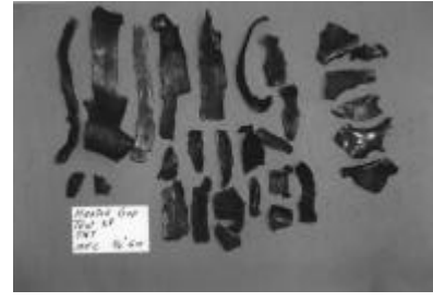
HGT-38. TNT, 0.75-inch gap, 100°C.
