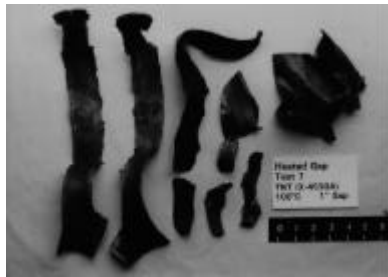
HGT-7. TNT, 1-inch gap, 100°C.
