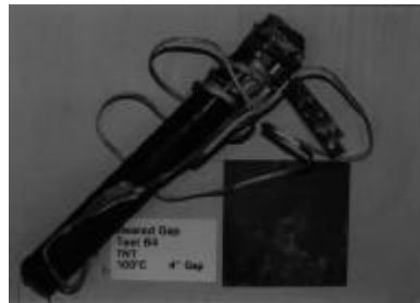
HGT-64. TNT, 4-inch gap, 100°C.
