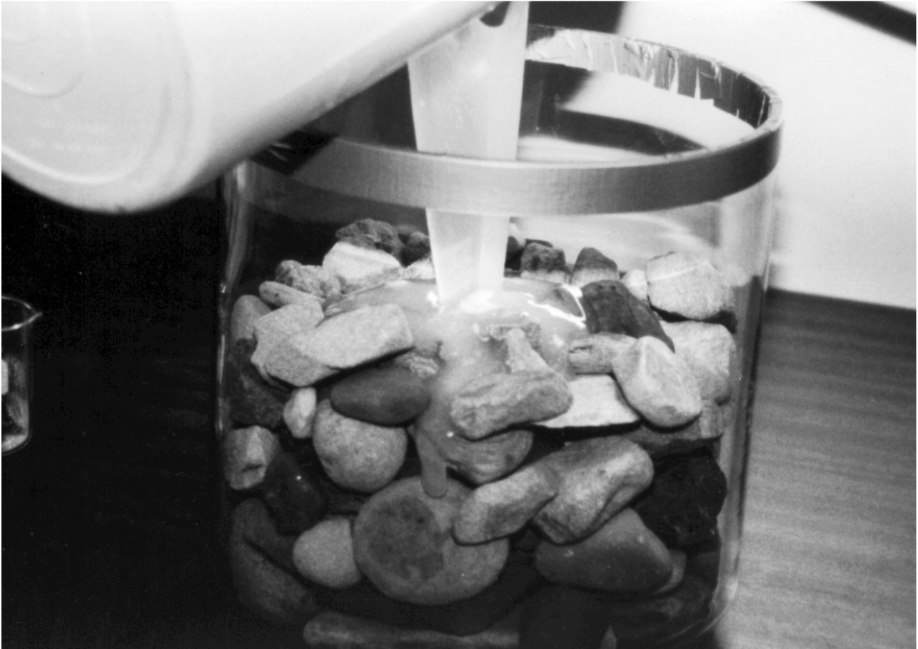
Figure 1.—Freshly prepared gel being poured into a jar containing rocks and coal dust.
