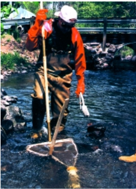
Collecting a macroinvertebrate kick sample from riffle substrate (USGS-NAWQA method).
