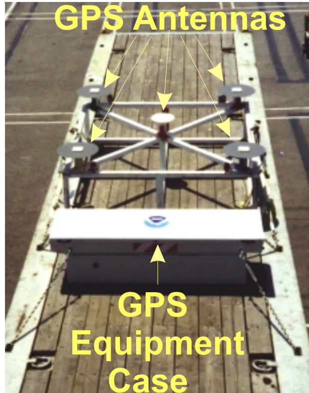
Figure 5 - Equipment used for GPS height and attitude measurement on an ATD.
