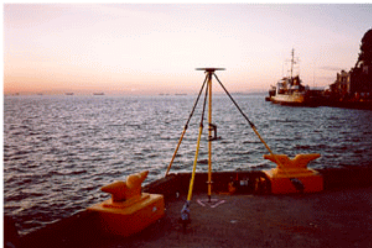
Figure 3 - Occupying tidal stations with GPS.
