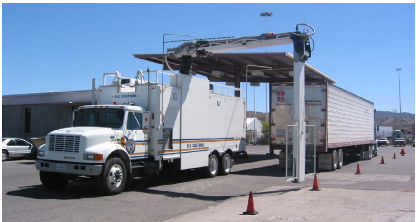
CBP mobile x-ray unit making an unintrusive inspection of a commercial vehicle in the commercial vehicle secondary inspection area. Mariposa POE. June 2003.
