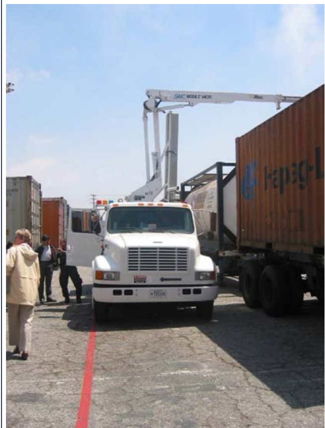
Mobile VACIS unit. The arm with the gamma ray sensor overhangs on the opposite side of the container and transmits images as the truck moves along the length of the containers waiting to be screened. Port of Long Beach. April 2003.
