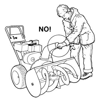
Most snow thrower injuries happen when consumers try to clear snow from the discharge chute or debris from the auger/collectors. Always stop the engine before attempting to clear snow and debris from any part of the snow thrower.
