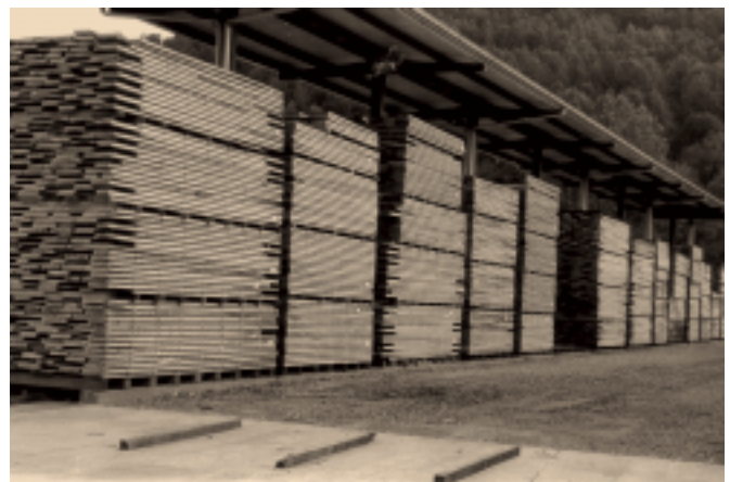
Figure 5.2—Air drying T-shed for hardwood.
