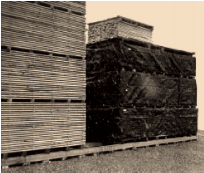
Figure 4.2—Good air drying yard: packages covered with plastic fabric to slow drying during dry and windy weather.
