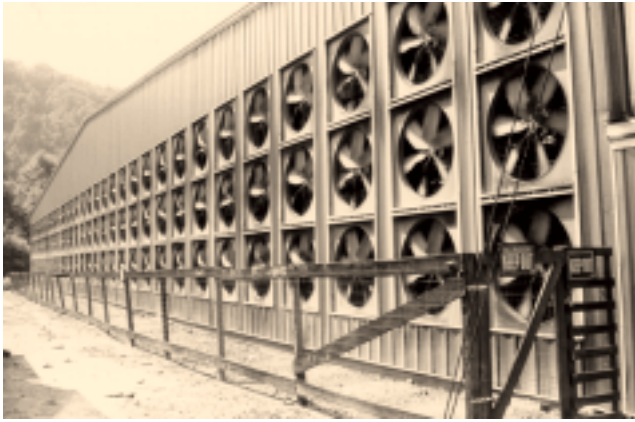
Figure 5.4—Typical fan shed used in a mill in Appalachia. Drying must be carefully monitored to prevent checking.
