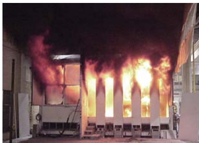
BFRL measured the thermal behavior of gypsum/steel wall assemblies subjected to severe fire conditions.
