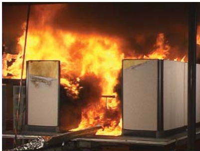
Photographs of the burning of a typical office workstation.
