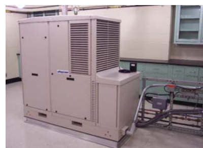
Residential fuel cell undergoing testing in a NIST laboratory.
