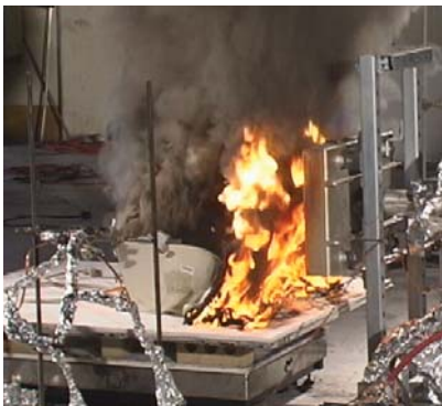
Computer monitor subjected to an external heat flux of 15 kW/m 2 .
