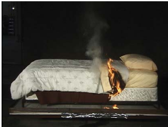
Bed at 1 minute after bed clothes ignition.
