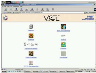
Left – the current VCCTL 4.0 interface, offering databases, cement hydration, and concrete property computations. Right – a sample of a cement microstructure, before hydration, from the current version of CEMHYD3D, the cement hydration module in VCCTL 4.0, which uses real cement particle shapes, sizes, and chemical makeup.
