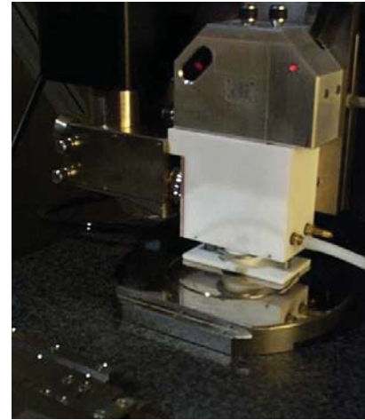
Figure 1: AFM humidity-controlled chamber.
