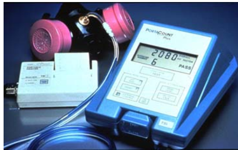
Quantitative Fit Testing using an Ambient Particulate Measuring Device
