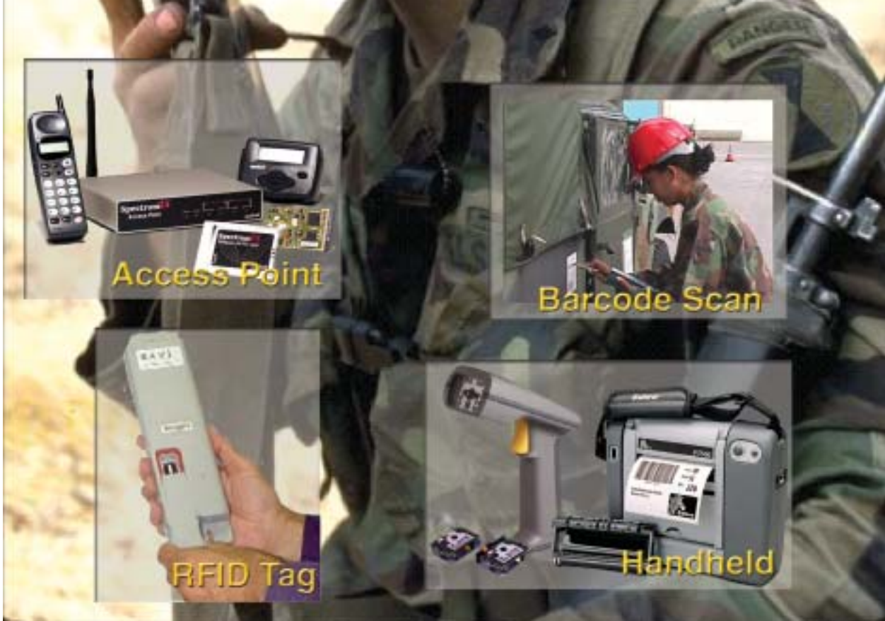
AIT hardware and software write the media, read the information stored on them and integrate that information with other data in logistics information systems.
