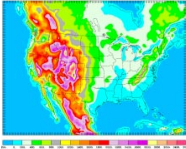
Fig. 1. Domain and terrain for the 40-km RUC-2. Topography is shown with 200 m contours.
