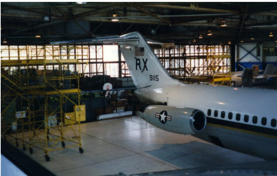
C-9 aircraft without fall protection for personnel who work on top of fuselage.
