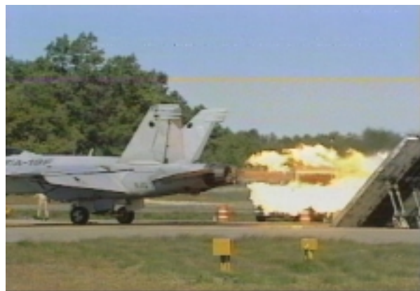
Super Hornet undergoing jet blast deflector and aircraft engine testing.
