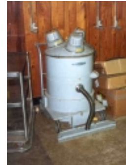
HEPA filter vacuum used to clean firing range floors.
