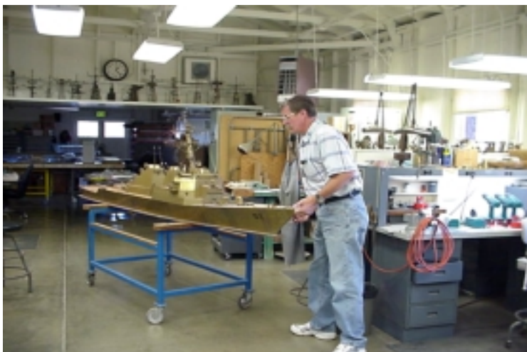
Model makers used unstable carts that were either too low or too high for workstation comfort
