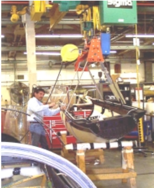
Flip-Rite positions aircraft canopy on sawhorses
