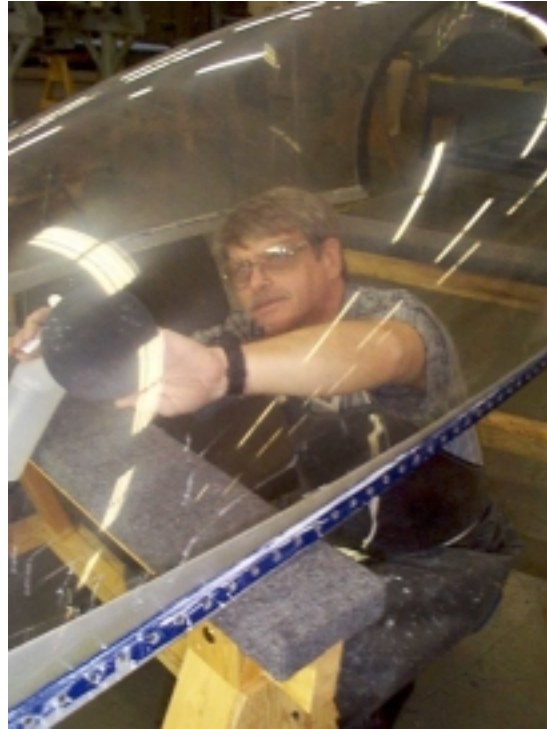
Mechanic having difficulty working on underside of canopy before ergonomic improvements
