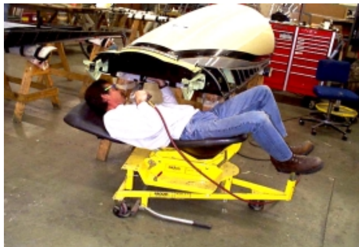
The tilting seat of the industrial positioner provides proper body support
