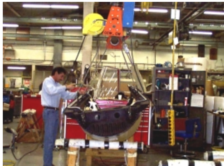
Flip Rite securely cradles an aircraft canopy
