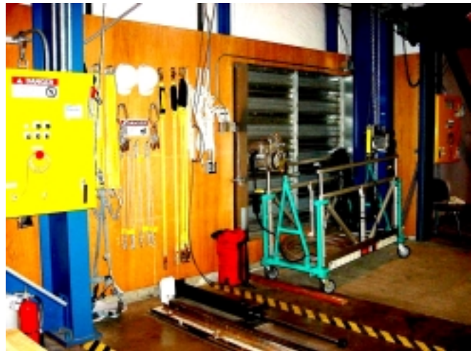
Fall-protection platform with fall-arrest lanyards
