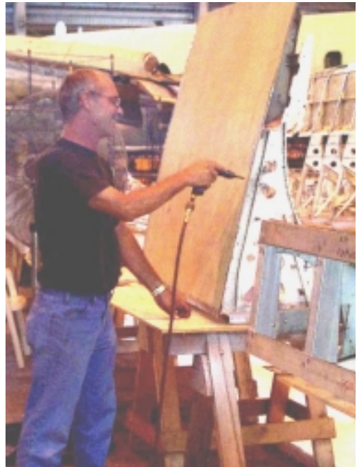
Mechanic works comfortably on flapwell mounted on flapwell fixture
