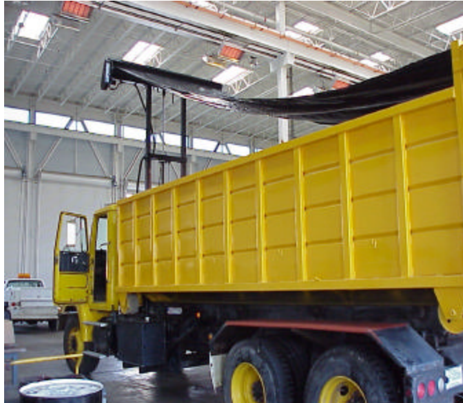
Ergonomic Improvement - Sky hook automatically covers load and eliminates risk of injury and falls
