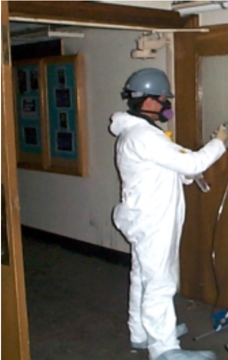
Navy industrial hygiene clearance sampling followed clean up of Pentagon after the terrorist attack
