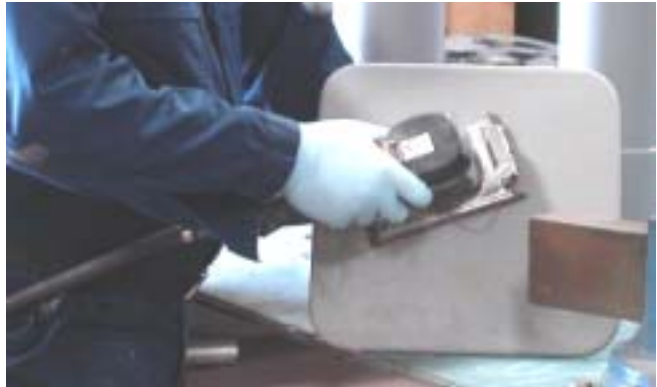
Anti-vibration jitterbug sander prevents HAVS and is most comfortable for SIMA's Antenna Shop.
