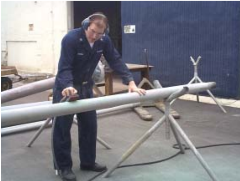
Antenna Shop personnel using a jitterbug sander that was not designed to be ergonomic or low in vibration to prepare an antenna for painting
