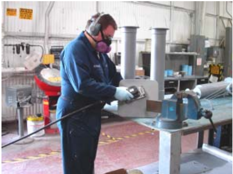
Worker uses the ergonomically designed jitterbug sander to prepare surface for painting.
