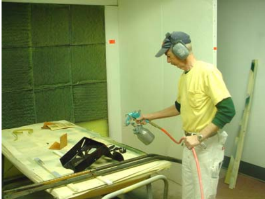
Enhanced ventilation system removes airborne hazards.
