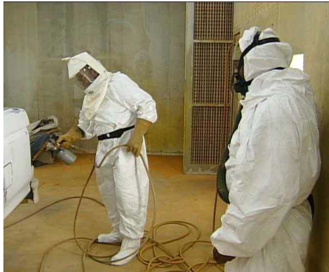
Painters in paint spray booth wear protective clothing and respirators to avoid contact with airborne contaminants.
