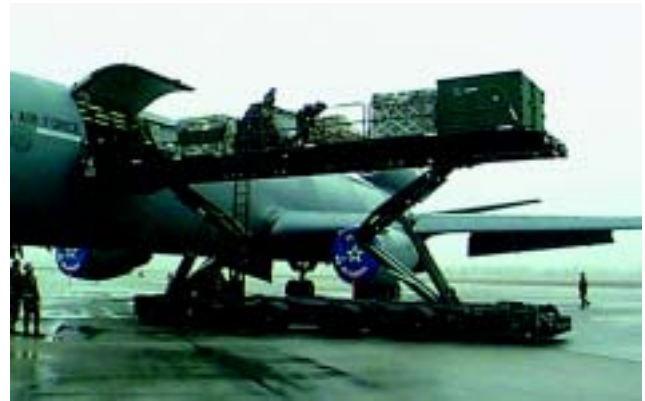
Thirty-eight Tunner aircraft loaders were used to move more than 53,000 tons of cargo during Operation ALLIED FORCE.
