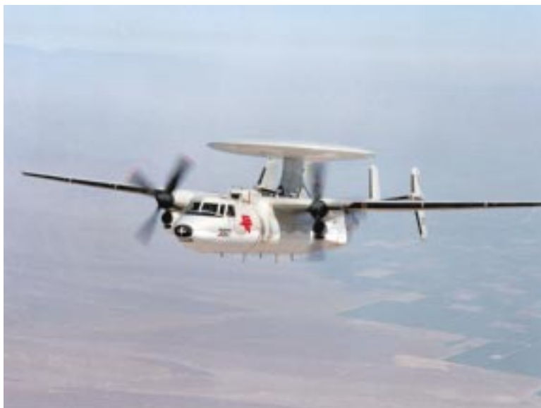
The E-2 Hawkeye is capable of detecting air and maritime targets and provides identification friend or foe link as well as HF, VHF, and UHF communications capabilities.
