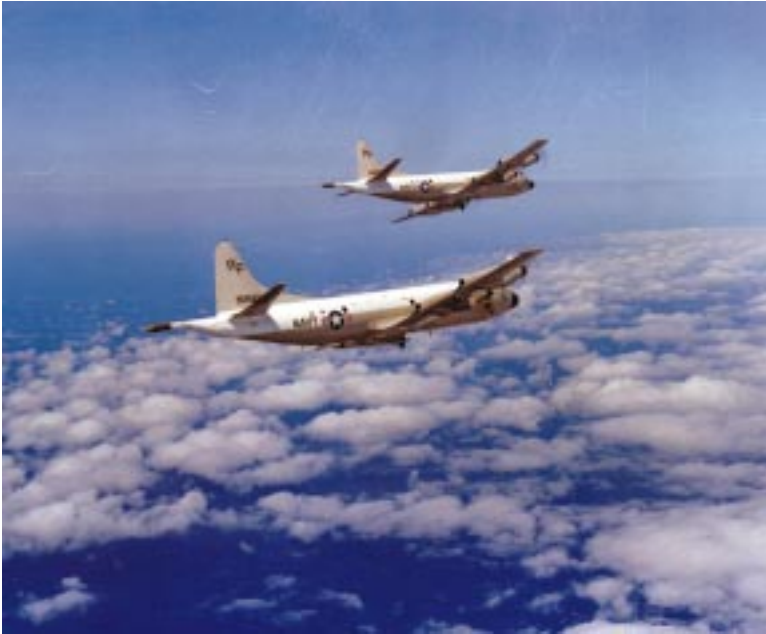
The P-3 aircraft provides maritime surface radar search, electronic surveillance, HF, VHF, and UHF communications. Some have been configured especially for the CD mission.
