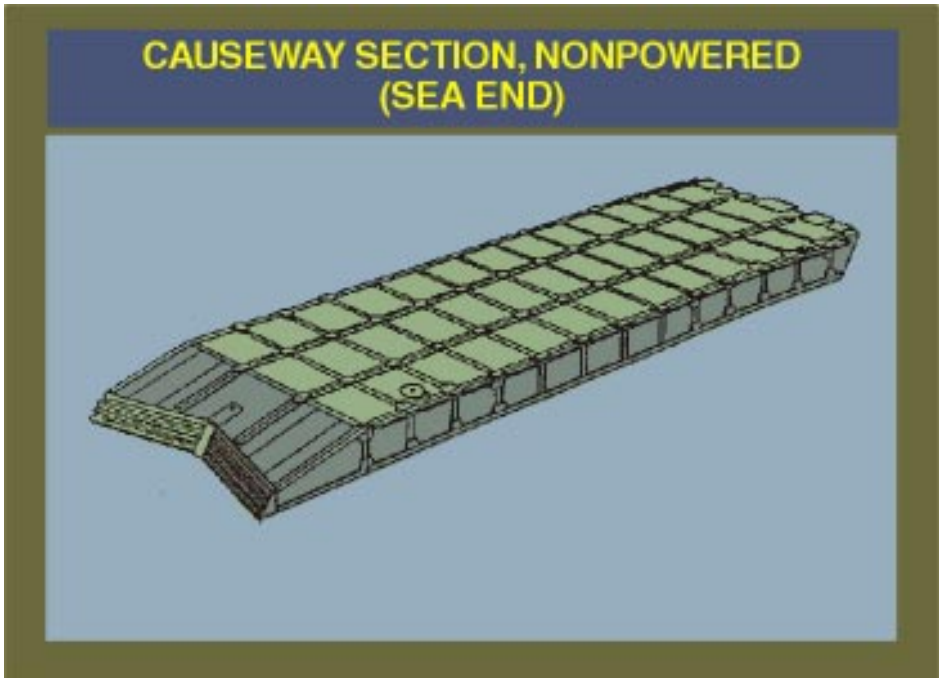
Figure IV-5. Causeway Section, Nonpowered (Sea End)
