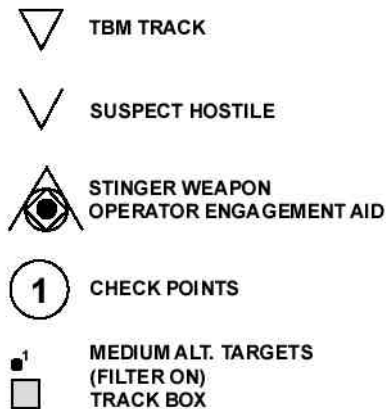
Figure 2-20. Remote Terminal Unit Symbology.
