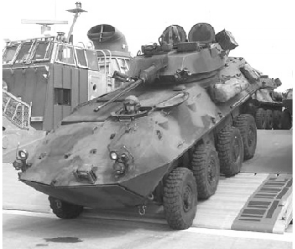
The Bison, a Canadian version of the eight-wheeled Light Armored Vehicle, being off-loaded from a ship.
