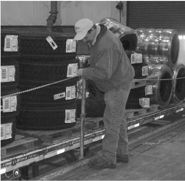
Mark Romanoski of DDSP places chains along a truck pit to guard against falls.
