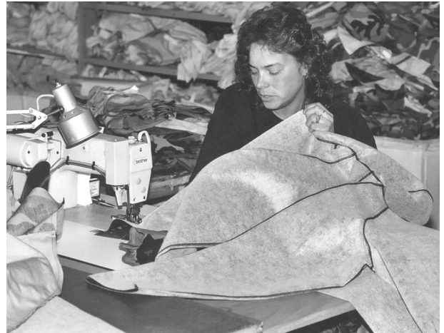
Sharon Stafford shown joining linings to outer shell of the JLIST chemical protective coats at Creative Apparel's plant in Harmony, Maine. The ensembles inner layer is designed to provide the user with protection from the effects of chemical and biological contaminants, and toxic industrial material in any form including anthrax, sarin gas and smallpox. (Photo by Frank I. Johnson, Jr.)
