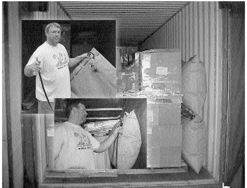
Craig George, DDSP, adds air to bags ready for sea transport to Germany. The air bags stabilize loads in place, reducing damage to the shipped commodities. (Photo by Maj. Mark Rivers)
