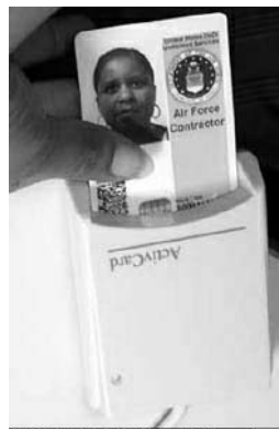
A user inserts her Common Access Card into a reader connected to her desktop computer. These cards will enable users to digitally sign as well as encrypt and decrypt e-mail. (Courtesy photo)
