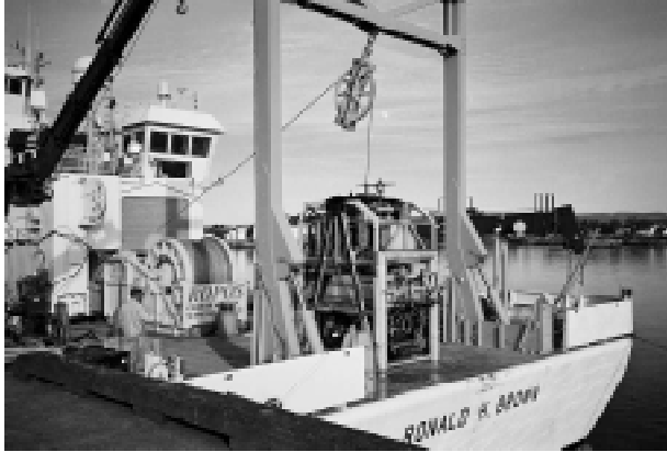
ROPOS remote operating vehicle on stern of NOAA RV Ronald H. Brown
