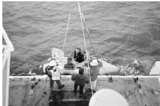
Lowering the ROPOS remote operating vehicle from stern of NOAA RV Ronald H. Brown (Photos courtesy of Jennifer Bloeser, Pacific Marine Conservation Council)
