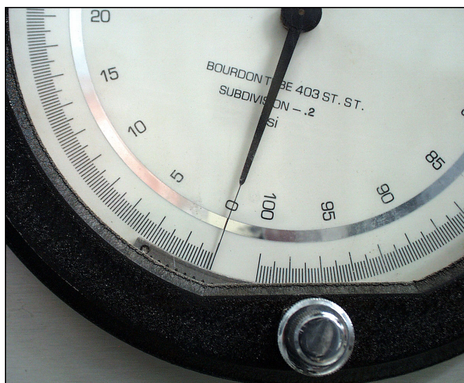
Figure 17 Properly Aligned CFO Pressure Needle Reading
