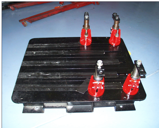
Figure 7 Mounting Feet Assembly
