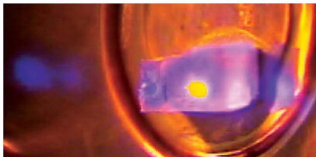
Figure 1: A 2,5 DHB single crystal on the sample stage. The bright yellow feature is the near UV laser spot. Notice the light pipe effect as visible radiation escapes from the ends of the sample. The sample is approximately 3 mm long.
