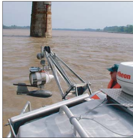
Figure 3. Use of a collapsible bag sampler on the Mississippi River at Thebes, Illinois.
