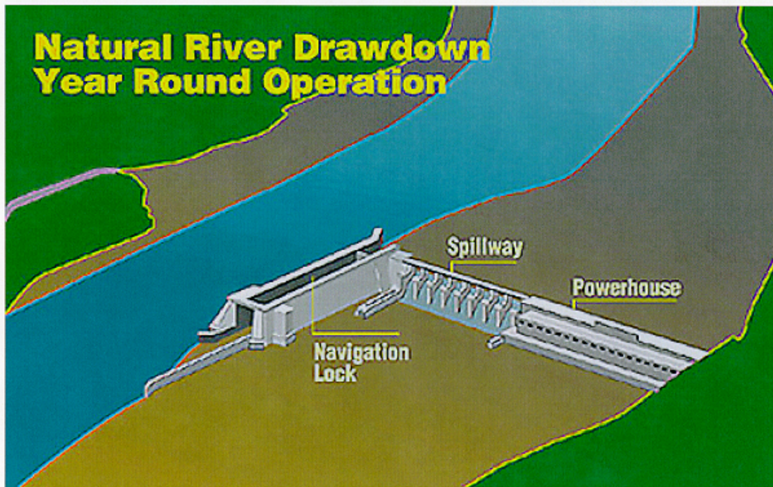
Figure 3-3. Conceptual View of Changes at a Dam with the Natural River Drawdown Alternative
