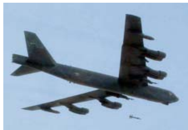
Barksdale AFB, LA—February 2003, a B-52 with the Litening II targeting pod drops a GBU-12 laser guided bomb during an operational utility evaluation. The integration of the targeting pod, originally scheduled for June 2003 was accelerated to improve the capabilities of combat B-52s to drop laser-guided munitions in Operation IRAQI FREEDOM.
