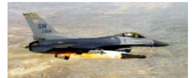
Air Force Test and Training Ranges "Vital National Assets"—An F-16 CJ pilot fires an AGM-65D Maverick missile at a target during an air-to-ground Weapons System Evaluation Program named Combat Hammer.
