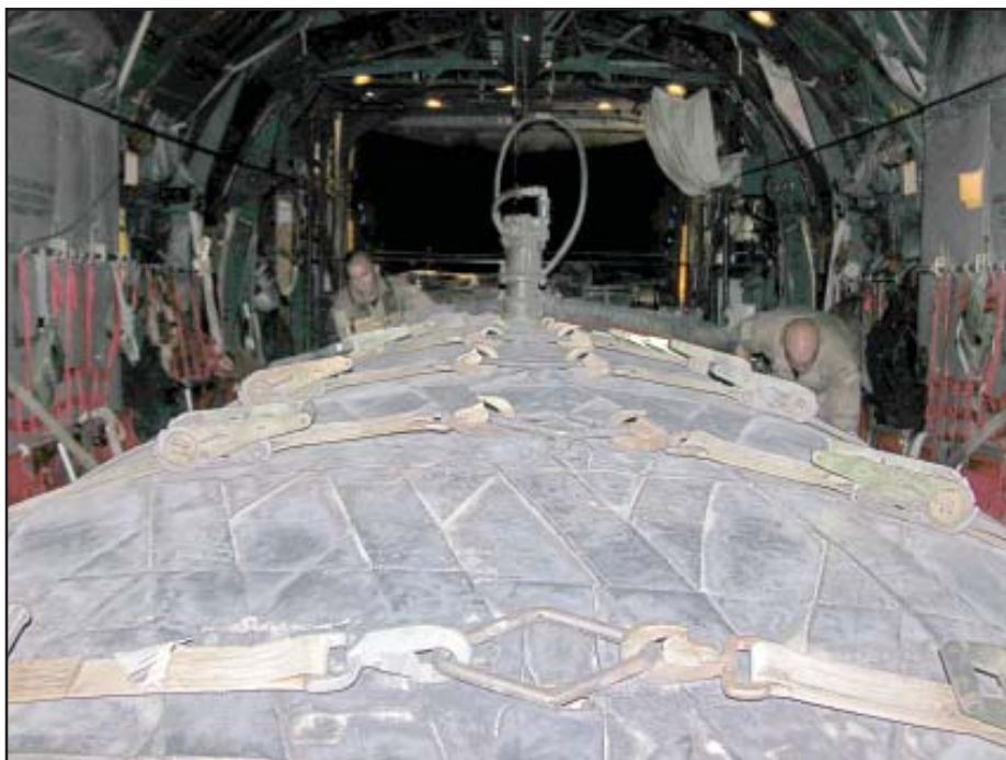
Staff Sgt. Chris Cooper and Senior Airman Pete Kaplan tighten straps on the 3,000 gallon fuel bladder before off-loading fuel at a forward deployed location.
