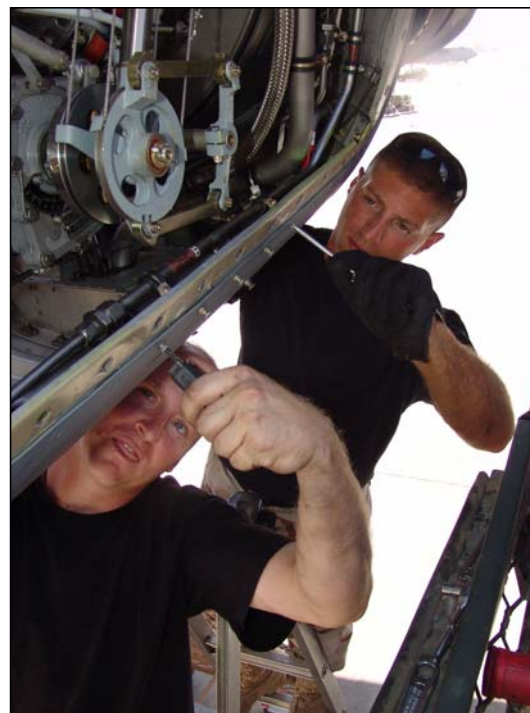
(Right) Senior Airman Nicholas Raia and Staff Sgt. Anthony Mobilian both 746 EMXS, engine mechanics, install an engine cowling.
