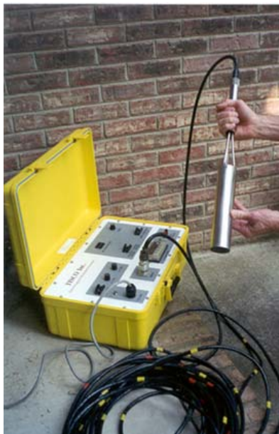
Figure 2: The Electromagnetic Borehole Flowmeter System
