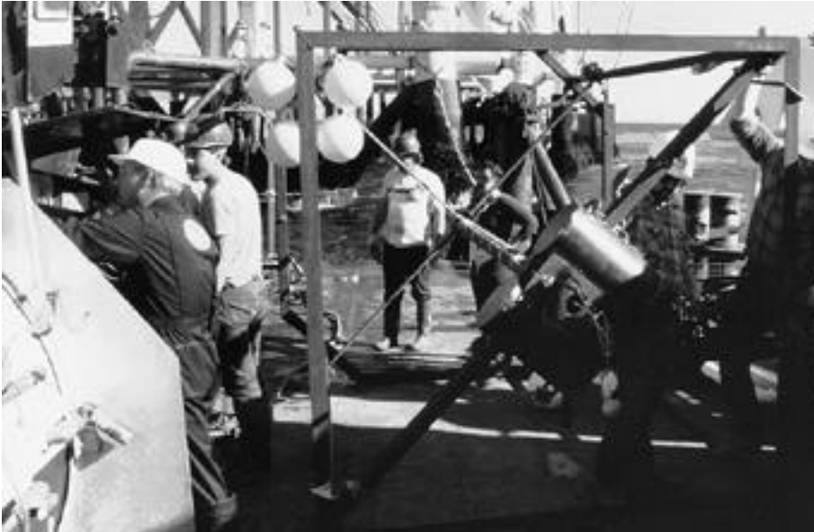
MMS places four strong motion instruments on sea floor in the Santa Barbara Channel to measure seismic activity.
