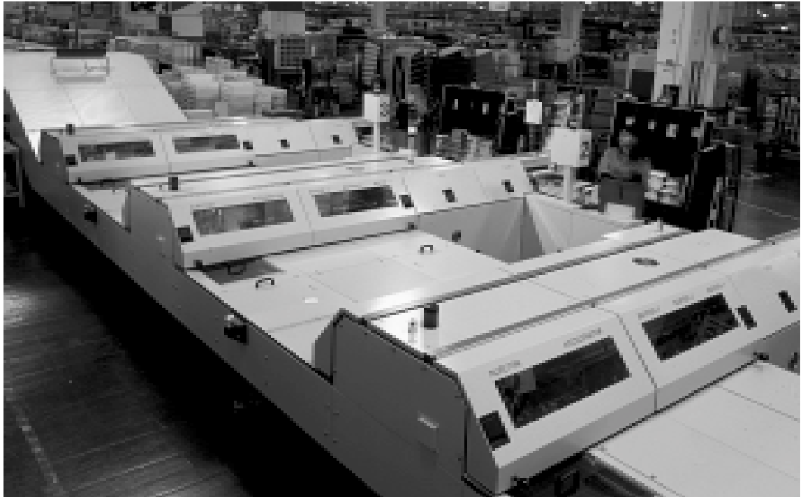
The Model 100 Automated Flat Sorting Machine will be used to test the preparation of flat-sized mailpieces on automated sorting equipment.
