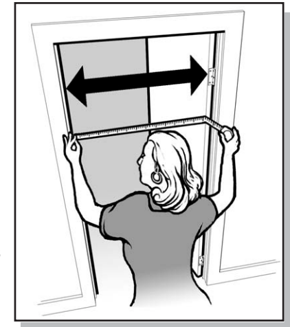
Measuring the clear opening from the face of the doorstop on the frame to the face of the open door
