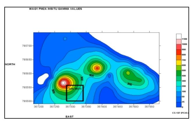
Figure 7. PM-2A radiation map generated from DART/M1 in situ gamma readings.
