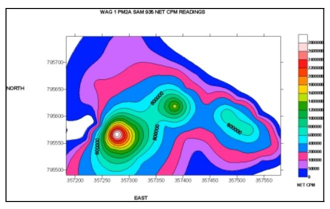
Figure 6. PM-2A radiation map generated from SAMS readings.
