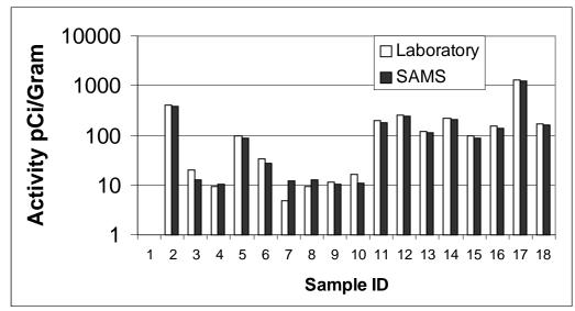
Figure 4. Comparison of SAMS and laboratory results.
