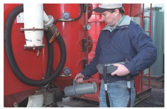
Figure 3. Radiation detection using the SAMS.
