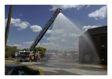
Figure 4-3. The Ladder Pipe Decontamination System (LDS)
