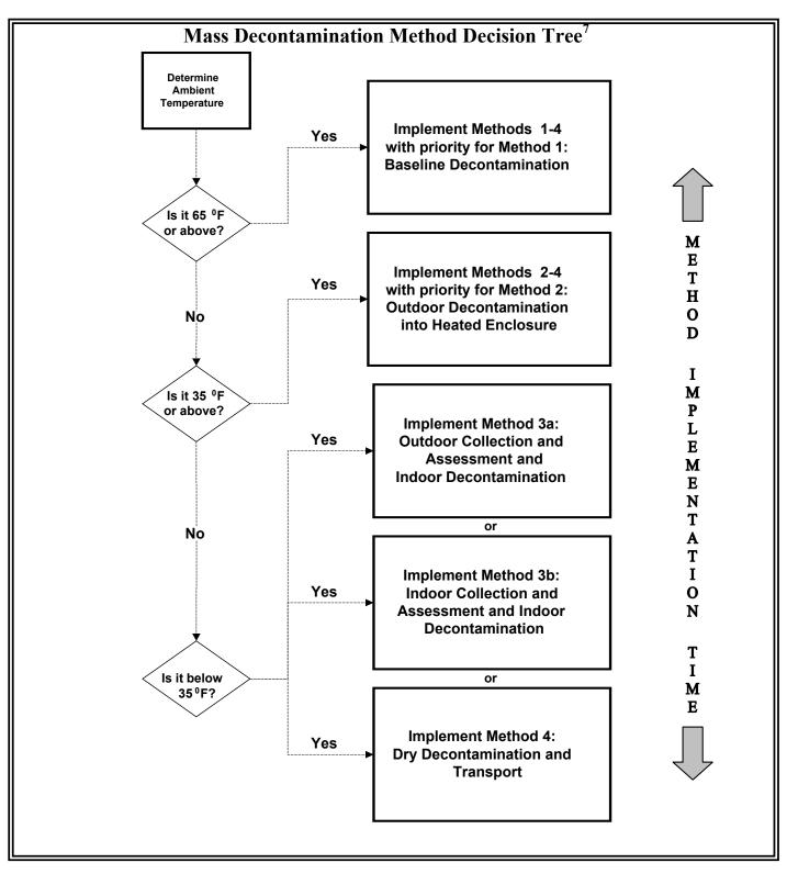
Figure 6-2. Mass Decontamination Method Decision Tree
