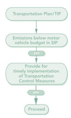
Figure 5: Transportation conformity process
