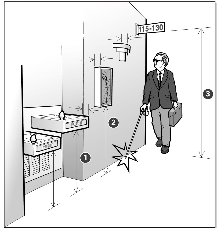
Overhead and wall-mounted objects that may be hazards along a pedestrian route.
