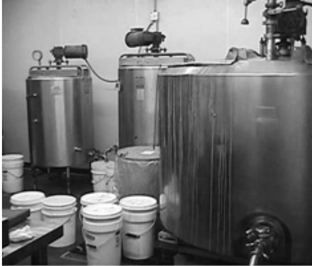
Figure 1. Mixing room, Case Cluster 1. The large mixing tank holds heated oil and butter flavoring mixture. Note loose-fitting lid, spillage on the outside of the tank, lack of local exhaust ventilation, and open 5-gallon buckets used to manually transfer concentrated butter flavoring from the smaller heated tanks to the large mixing tank.
